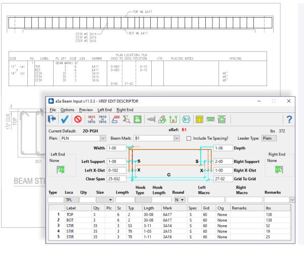
Powerful detailing tools like aSa Beam (left), Linear, Circular Area, Slab, and others automate bar development, eliminating the need to manually draw bars and type each item's callout.
