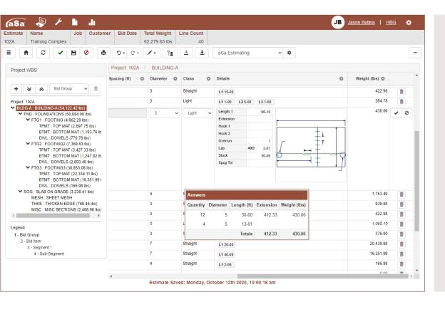
Estimating has built-in tools to calculate linear steel, varying bars, circular areas, ties, and other structure types. The Answer Window updates in real-time as you enter material, helping you to catch and eliminate mistakes.
